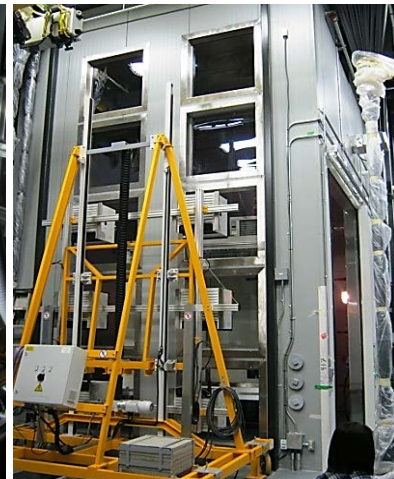
Figure 3. Concordia mobile solar simulator with the two-storey high environmental chamber.
