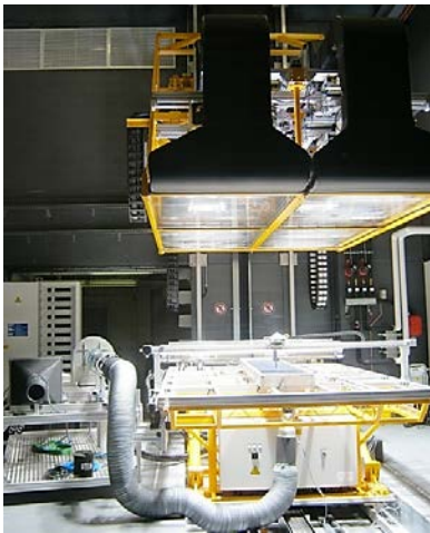
Figure 1. Concordia solar simulator testing BIPV/T air collector in horizontal position.
