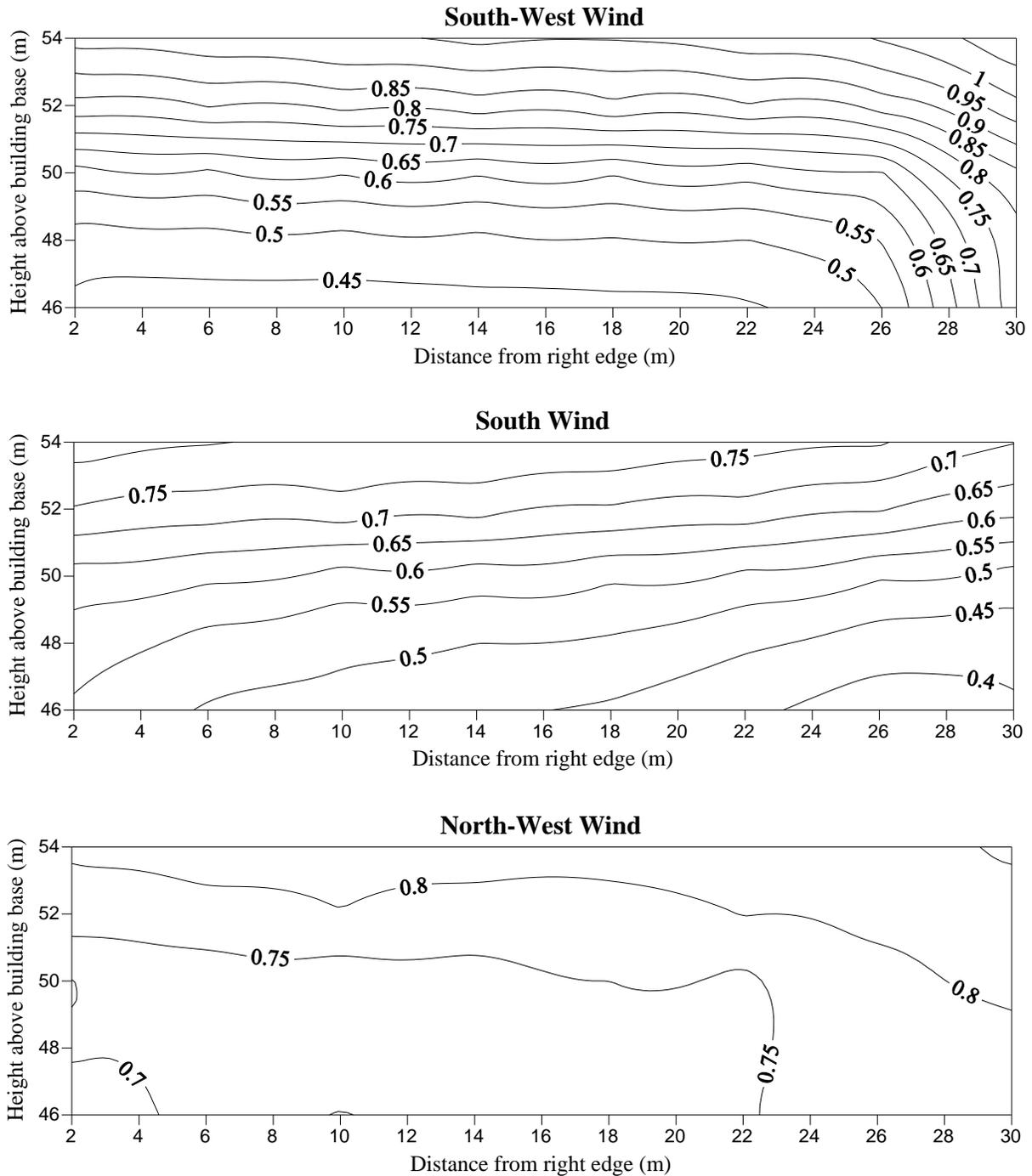
Figure 4: Distribution of  $V_{loc}$  (as a fraction of reference speed) over the UTC surface
