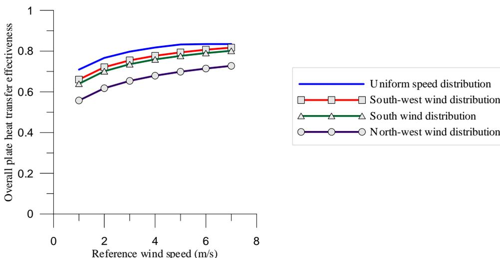
**Figure 7: Comparison of  $\epsilon$  for different wind speeds and directions**
