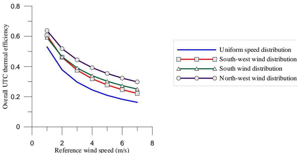
**Figure 8: Comparison of  $\eta$  for different wind speeds and directions**
