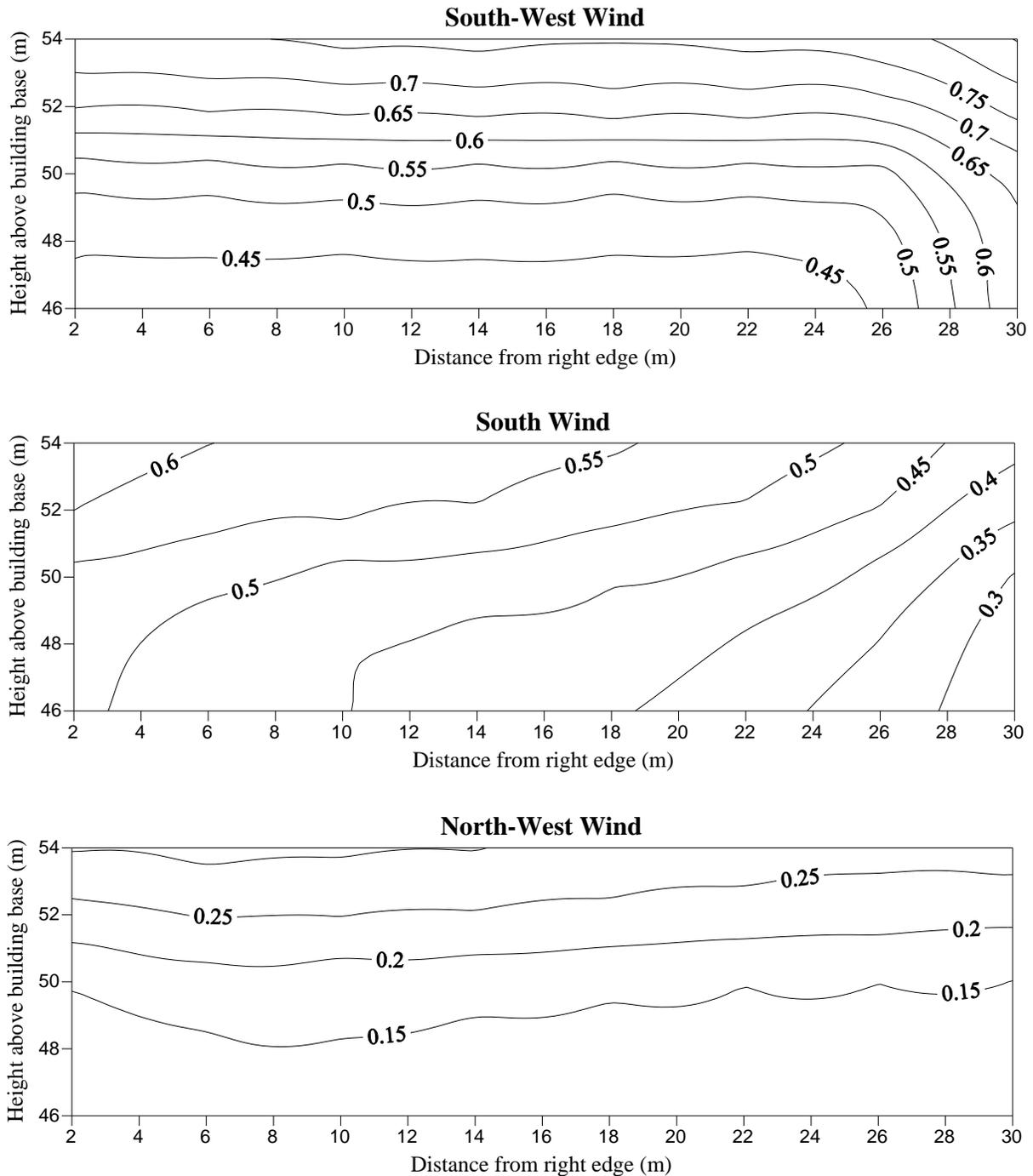
**Figure 6: Distribution of  $V_{normal}$  (as a fraction of reference speed) over the UTC surface**
