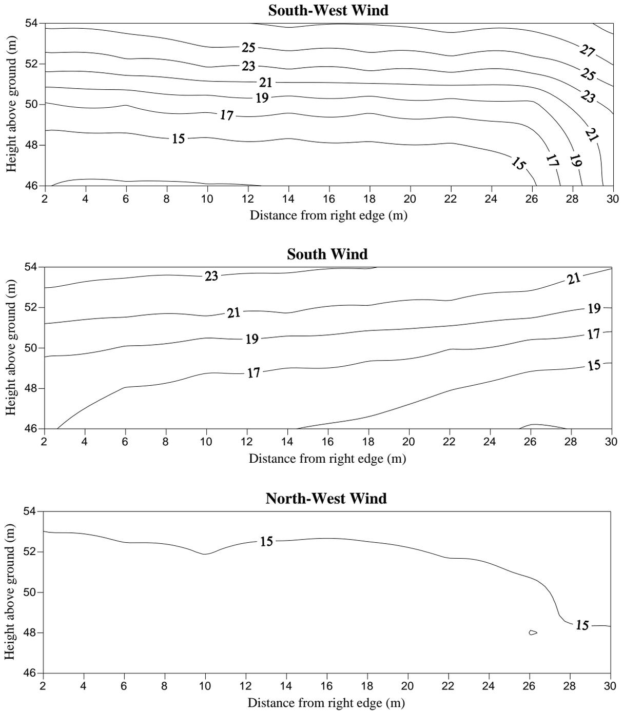
**Figure 5: Distribution of CHTC ( $W/m^2K$ ) over the UTC surface for a reference velocity of 3 m/s in full-scale**
