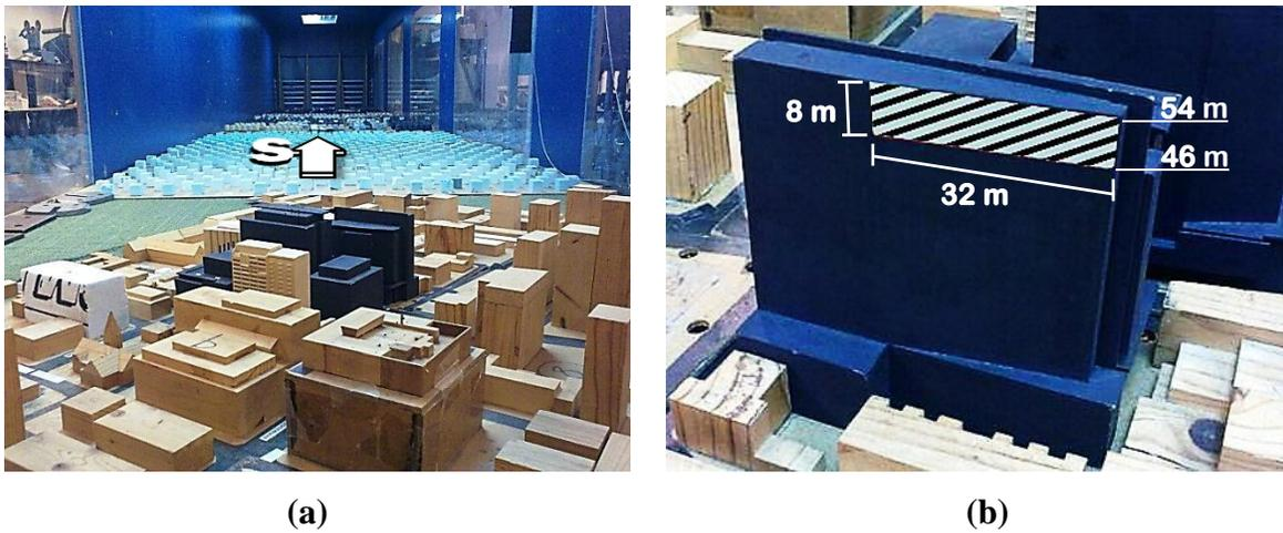
**Figure 1: (a) Test building, surroundings and roughness models placed in the wind tunnel; test wind direction - South (b) Model of the JMSB building with BIPV/T location hatched**
