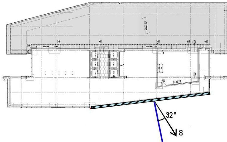
**Figure 2: Schematic plan of the JMSB building showing the orientation of the BIPV/T wall**
