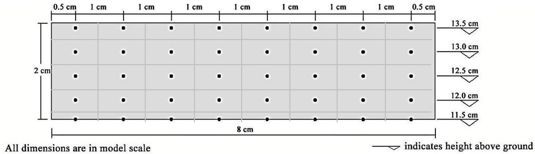
**Figure 3: Schematic of the BIPV/T wall showing the positions of velocity measurement points**
