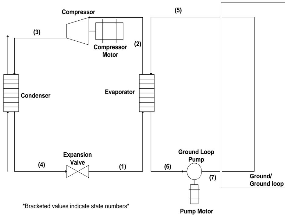
**Figure 1: System diagram of heat pump system 1**
