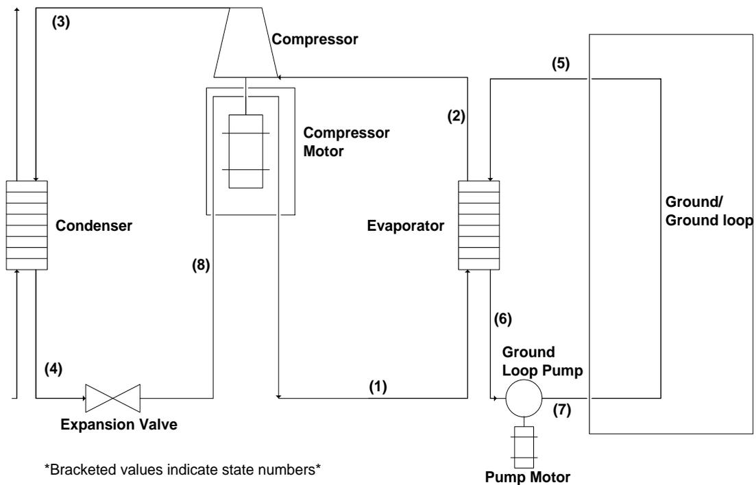
**Figure 2: System diagram of heat pump system 2**
