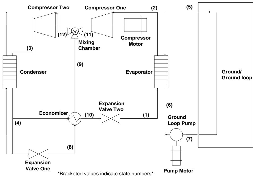
Figure 3: System diagram of heat pump system 3
